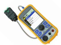
The MT-H9000 training simulator comes with an EOBD Scan tool for reading parameters and faulty codes. **EXXDTEST**® CL550, multi-functions tester bringing together the functions of Oscilloscope, Multimeter and OBD II scan tool.
