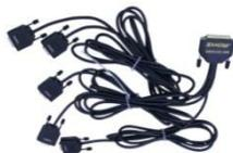
**AMUX-C4C-DB9:** 2 m twisted cable with DB25 to 4 x SubD9 (CAN channels)
