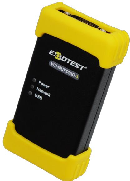
The **VCI-MUXDIAG-3** is a compact multi-protocol communication interface particularly suited to the analysis and diagnosis of the electronic architectures equipping the most recent vehicles and mobile machines.
