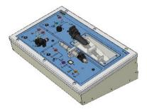
Module DT-C002 lets trainees acquire skills and expertise in injection and ignition technologies. The module facilitates this learning by allowing the trainee to control a pencil coil, a traditional petrol injector and a piezoelectric diesel injector.
