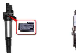
Use of a pencil coil-type ignition coil developed for the EP6DT engine. PSA wiring diagram
