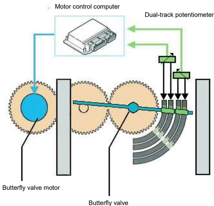
The position of the butterfly is determined by the motor action, which is controlled by the calculator.
