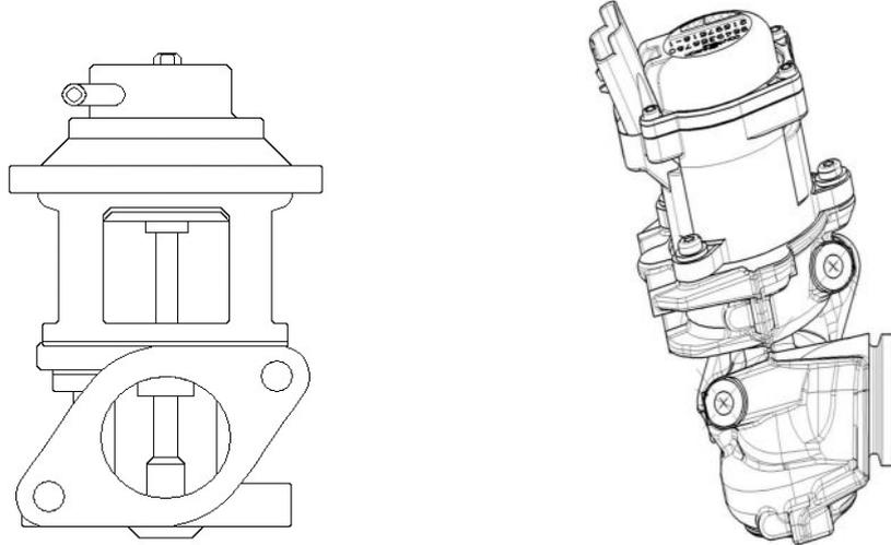
Whatever its type, the recycling valve is connected to the exhaust manifold.
