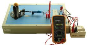
The sensor must be powered by the electronic control unit and the target rotated to alternate the magnetic poles.
