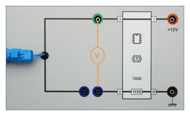
To wake up and deliver a signal once again, the sensors must detect six rising edges. They are energised with +12 V power.
