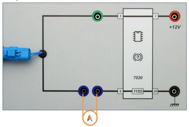
Given the reading track design (alternating pattern of north and south poles), a rectangularwave signal varying between 7 and 14 mA is recorded. The frequency of this signal represents the speed of wheel rotation.
