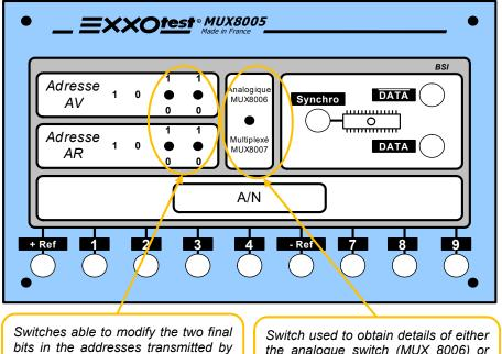
bits in the addresses transmitted by the BSI to the front/rear light receivers
