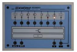
2- The MUX8004AR module detects that no information is being received from the BSI and switches to downgraded mode: the parking lights are turned on after 2 seconds.
