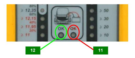
The green LED «OK» (12) lights up after connecting to the vehicle if the memory protection battery integrated in EXXOtest MI250S is correctly charged. The memory will be kept **for 2 minutes maximum**.
