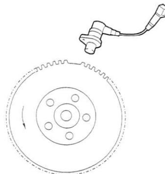
The sensor emits an electrical signal when a tooth of the flywheel passes by (magnetic field modified).
