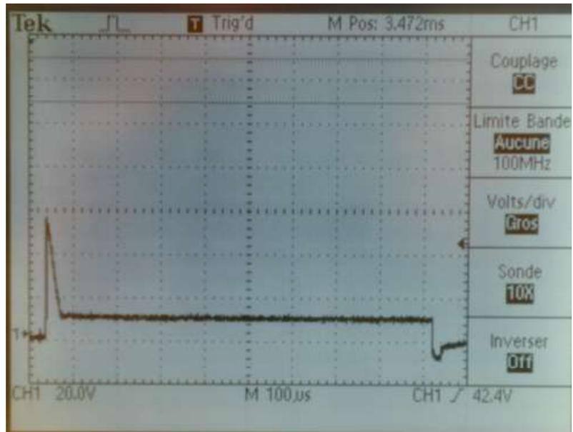
Capacitor charge with repeated 12 volts supply
