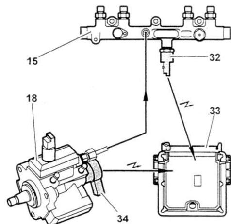
If the computer is unable to obtain the required pressure in the injection rail, the computer will record a "high pressure control" defect.
