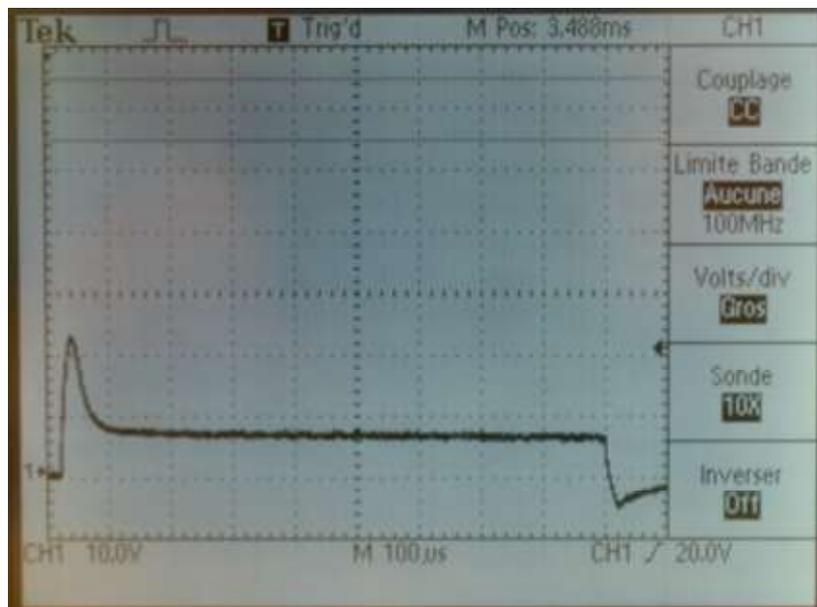
Details of capacitor charge:
