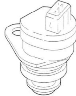
This sensor is based on "Hall effect" with 5 reference points per rotation.
