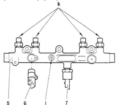
The high pressure injection rail is in forged steel.
