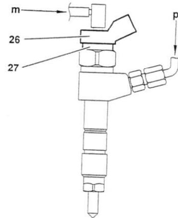
The injectors include several holes, promoting the spraying of the air/fuel mixture. They are adapted to the engine version, e.g.: 5 holes with a diameter of 0.16mm, (or 5 x 0.2 mm or 6 x 0.15 mm).
