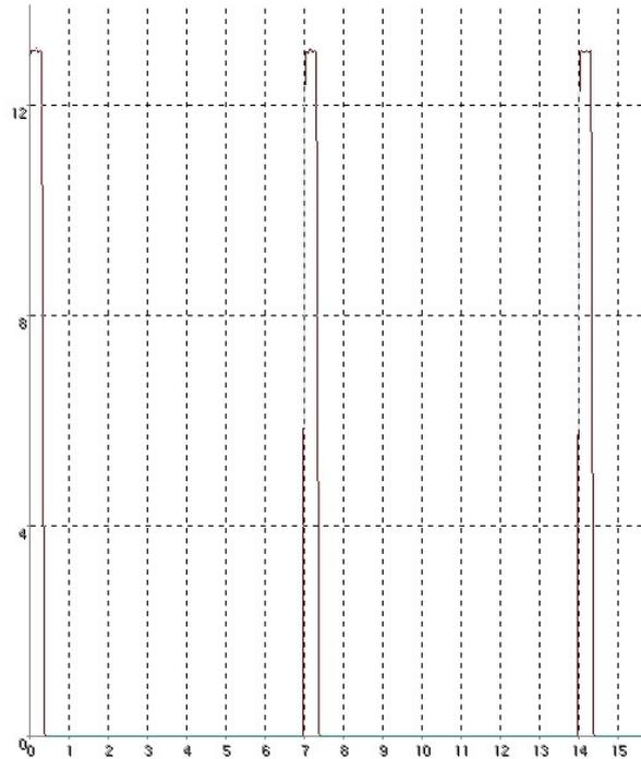
**CURVE 9: panel engine speed command output at terminal 62**
