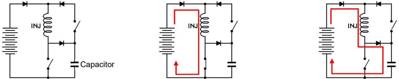
During injections, the capacitor discharges a short-term voltage of 80V into the winding, rapidly establishing a high current and therefore opening the valve rapidly.
