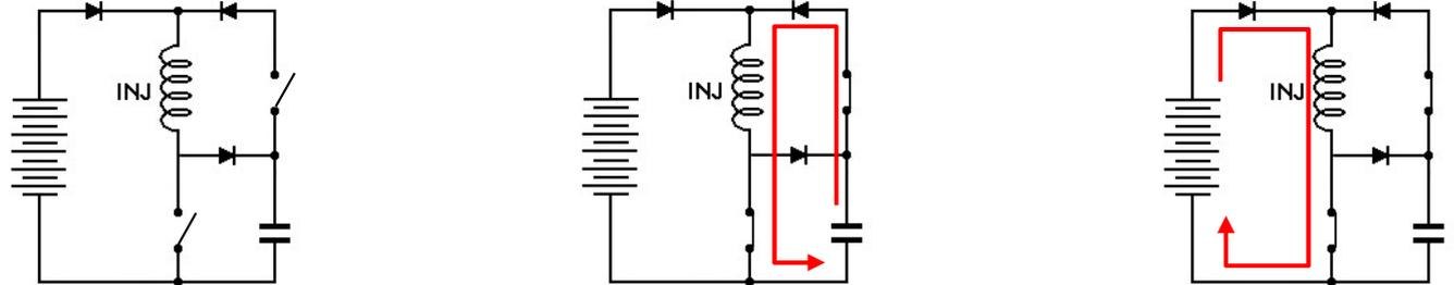
Maintaining current in the injector (with control)
