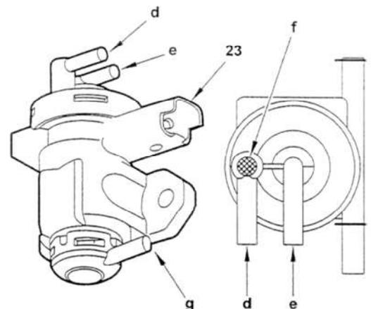
The solenoid valve connects the vacuum pump and the recycling valve capsule for exhaust gases (EGR valve).
