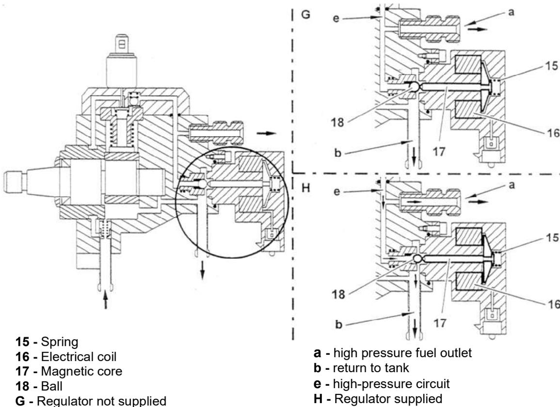
The high-pressure fuel regulator includes two pressure control circuits:
