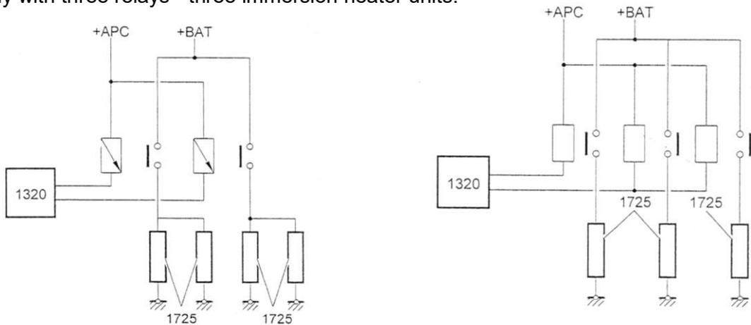
Assembly with two relays - two immersion heater units:
