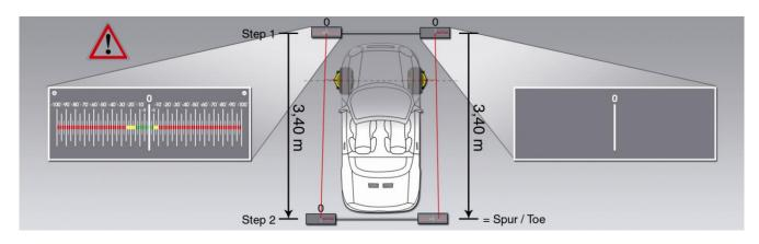
Move the toe target back by 3,40 m (Step 2)
