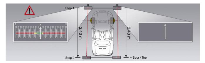
Put the toe target bar 3,4 m back and move it to "0" on the left hand side of the car (Step2).
