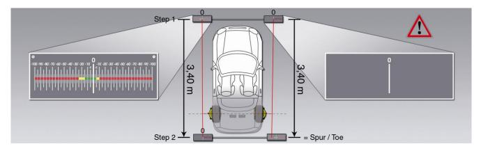
Adjust the toe target bar so the both sides show "0" (Step 1)
