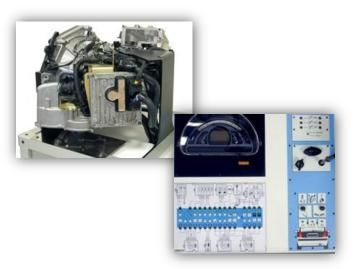
This simulator consists of an aluminium frame on caster wheels with a manual gearbox mounted on a metal frame.
