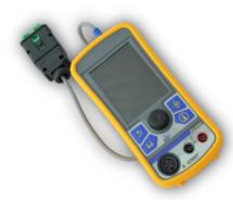
As an option you can use with this teaching model our EOBD Scan tool for reading parameters. **EXXITEST**® CL550 - multi-functions tester bringing together the functions of Oscilloscope, Multimeter and OBD II scan tool.
