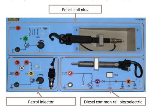
The cables' sockets placed on the face panel allow to execute assemblage of various elements easily and to control them like in real vehicle.
