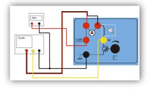
Injector assemblage schema allows to execute functionality of the injector and to boost voltage S2 as well as power at the injector coils. It gives the possibility to manipulate the speed and to understand the functioning of the injector.
