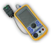
As an option you can use with this teaching model our EOBD Scan tool for reading parameters. **EXXIITEST**® **CL550** - multi-functions tester bringing together the functions of Oscilloscope, Multimeter and OBD II scan tool.
