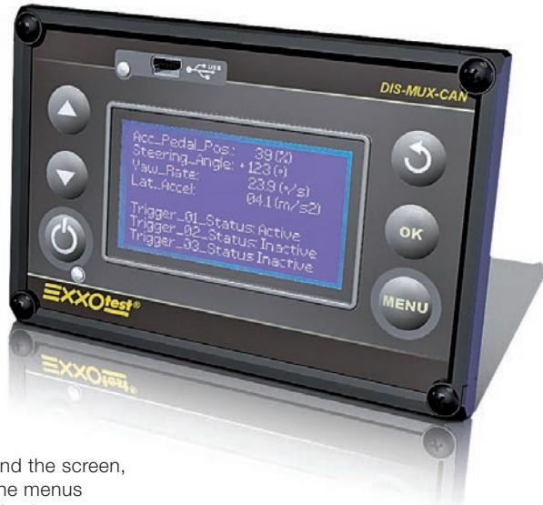
6 buttons placed around the screen, allow navigating into the menus of the embedded application as to select signals to be displayed.
