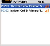
Throttle/Pedal Position Sensor/Switch B Circuit High Input
