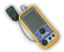
As an option you can use with this teaching model our EOBD Scan tool for reading parameters.
