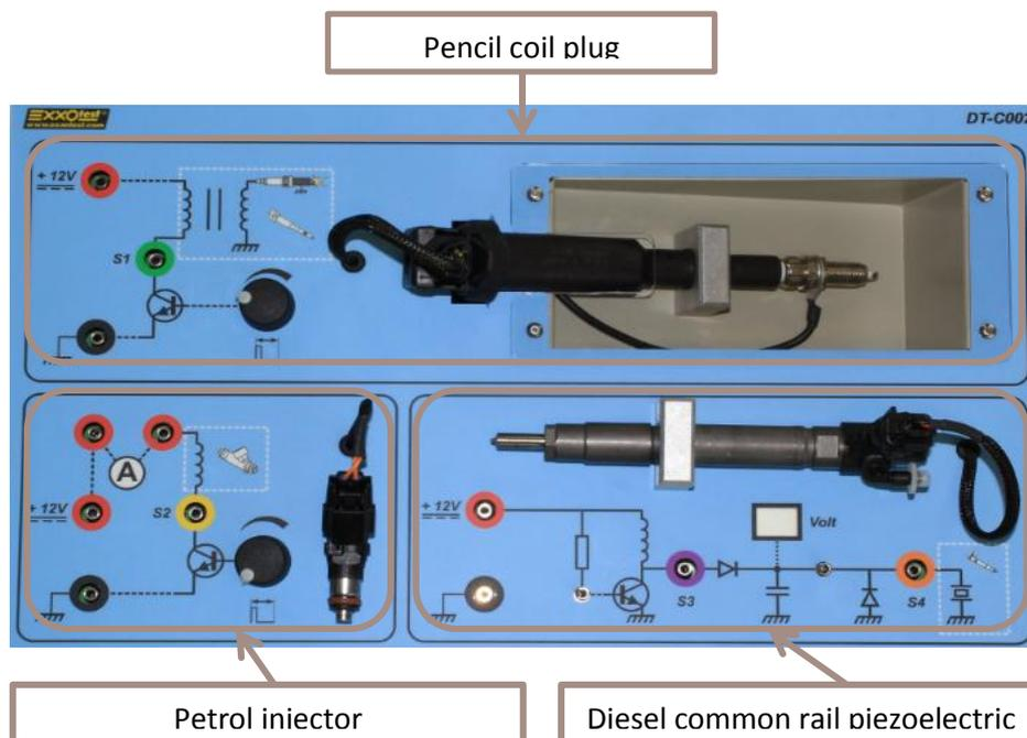
The cables' sockets placed on the face panel allow to execute assemblage of various elements easily and to control them like in real vehicle.
