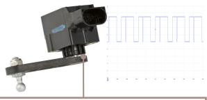
Analogue and digital sensors of the vehicle body's height
