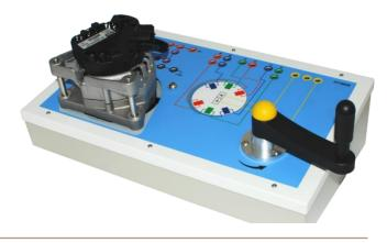
The DT-M008 introduces the technologies used by vehicle's alternator. This model gives the possibility to discover the energy transformation process (mechanical energy into electrical energy). It also allows the measurement of alternating current or rectified current (star, triangle and Diode Bridge).
