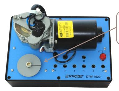
Window on the motor reduction gear unit shows the arm automatic return position system and the park system.
