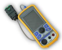
The MT-E5000 training simulator comes with an EOBD Scan tool for reading parameters and faulty codes. **EXXIDTEST**® CL550, multi-functions tester bringing together the functions of Oscilloscope, Multimeter and OBD II scan tool.
