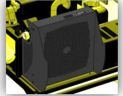
The cooling system, placed at the front of the chassis, includes the radiator, the fans unit, various hoses and an expansion bottle.
