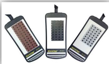
Another solution for analysis and diagnostics of engine system are the **breakout boxes**. Easy to use, they cover a large range of current automotive connectors. Each breakout box fits with the car manufacturer cable sections standards and therefore generates no disturbance on the vehicle. Measurements are done using delivered test leads. For the **EXXOTEST**® MT-Moteur-iDT-BSI you can use the **EXXOTEST**® MT-MOBM-EVIDTE3C.
