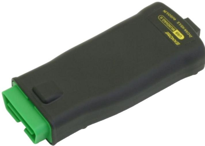
The USB-MUXDIAGII allows to interface a PC (or a pocket PC) with the CAN and KWP2000 diagnostic channels of a vehicle using an USB link.
