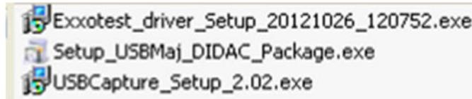
But before connecting the device to a PC using the USB cable supplied, you need to install the device driver. To do so, double-click the file 'Exxotest\_driver\_Setup....exe'.
