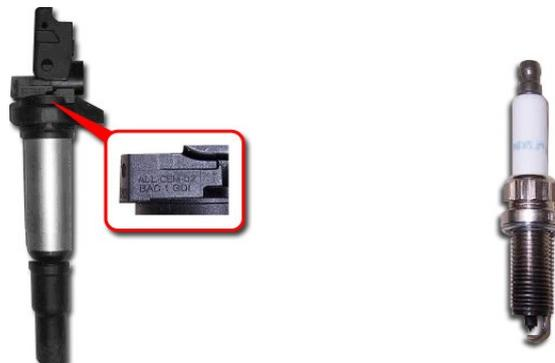
Use of a pencil coil-type ignition coil developed for the EP6DT engine.
