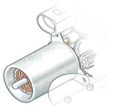
Note: As idling control is also done by this motor, the idle regulation solenoid no longer exists.
