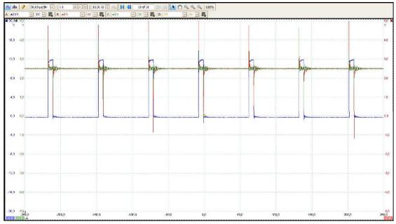
H. Determine the duty cycle percentage needed to be in the same case as above. The period is approx. 70  $\mu s$
