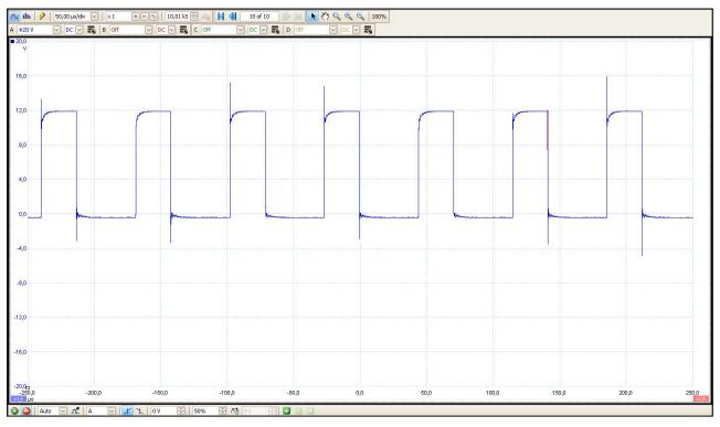
**E.** What is the duty cycle % in this position? The period is approx. 75 μs The control time is approx. 25 μs.
