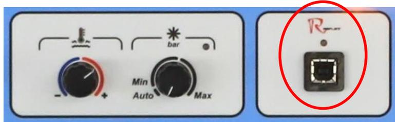
The LED above the USB plug on the model lights up blue when the cable is connected to the computer and flashes when the model is dialoguing with the REFLET software (data exchange).
