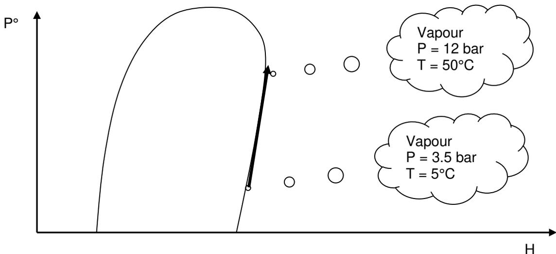
Condenser: The condenser is a heat exchanger. When the vapour enters the condenser, it changes state. The vapour liquefies at constant temperature, reducing its enthalpy, and transferring the heat (absorbed in the evaporator) to the air pulsed by the powered fans, until complete liquefaction.
