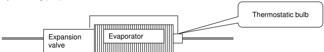
The system is designed to superheat the fluid by 5°C to 10°C at the compressor inlet. This increase in temperature is measured by the thermostatic expansion valve and controls the opening of this valve to ensure that the fluid is 100% gaseous when leaving the evaporator.
