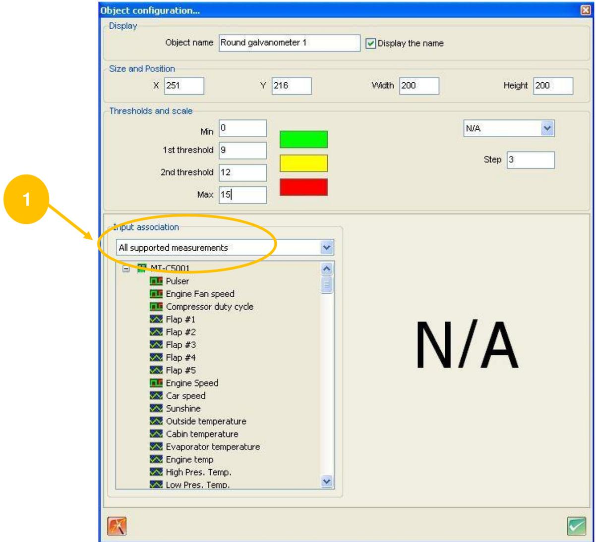
You must then select "Defined by the user" from the Unit and measuring **type section** (ID 1 above): you will only be able to access all of the signals proposed by the MT-C5001 model after this selection process.
