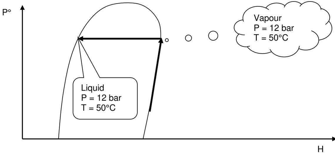
Thermostatic expansion valve: This device expands the fluid in the evaporator. It adjusts the flow depending on the temperature at the evaporator output, thereby controlling the complete evaporation of the fluid
