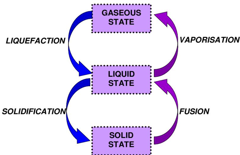
Enthalpy characterises the amount of heat contained in the fluid. The zero point of this scale corresponds to absolute zero. Variations are shown by the double arrows quantifying the additional energy the fluid requires to change temperature or state. Variations in enthalpy occur during the following two transformation phases: Sensible heat (variation in fluid temperature due to the contribution of heat) and latent heat (change in fluid state due to the contribution of heat).
