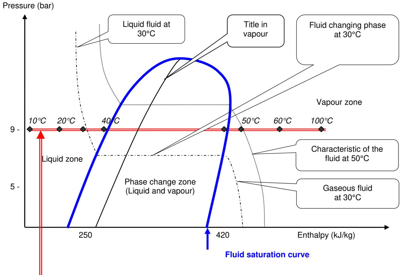
**Isobar straight: quantify the energy required to change the phase or temperature of a mass of fluid.**
