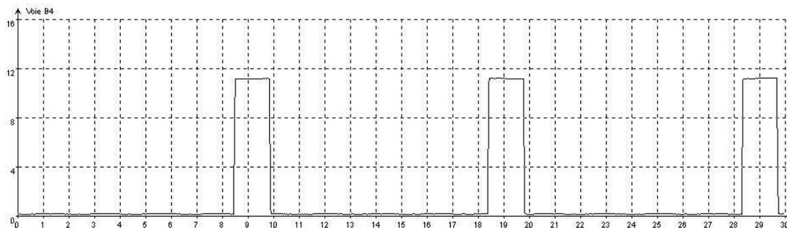
Electronic throttle control on accelerating to 100%.
