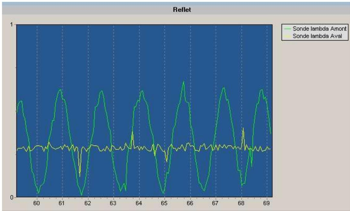
Operation with catalytic converter failure.
