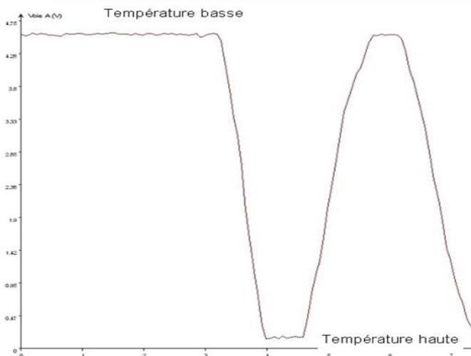
*It can be seen from the curve that resistance decreases as the temperature increases. It is therefore an NTC (negative temperature coefficient) thermistor.*
