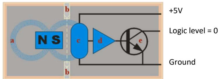
When the target passes between the magnet and the wafer, it is no longer subjected to a magnetic field and no longer delivers a signal. The transistor is blocked, the output logic level switches to 1.
