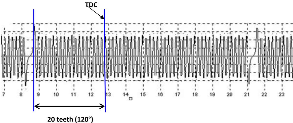
8. Using the signal transmitted by the engine speed sensor, determine the frequency with which the pulses caused by the target teeth occur for an engine speed of 3500 rpm
