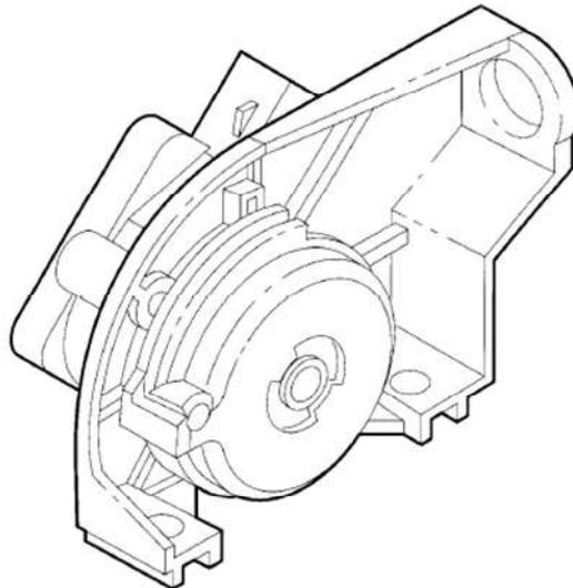
It receives a 5 V supply from the ECU and transmits to the ECU two variable voltages reflecting how far the accelerator pedal is depressed. One of these voltages is twice the other.
