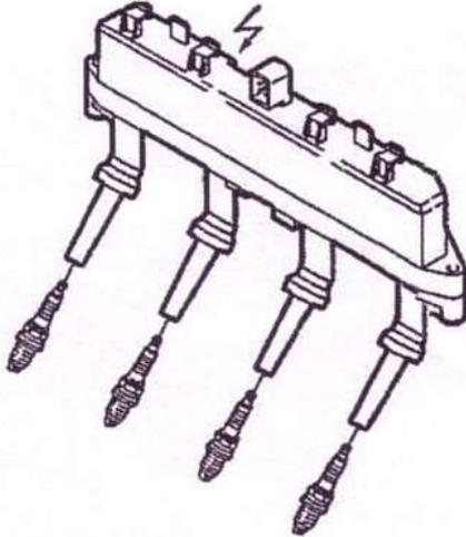
The ignition is of twin static type with a compact coil unit and no high-voltage leads. The compact coil unit comprises two coils with high-voltage outputs located directly above the spark plugs. Each coil comprises a primary winding linked to a secondary winding. Each secondary output is directly connected to a spark plug. This technology improves ignition quality.
