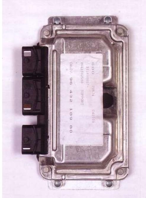
*The ECU is equipped with a 112-pin connector.*
