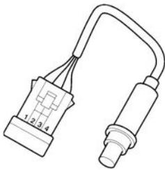
*The oxygen sensor measures the oxygen content of exhaust gases and transmits the information to the ECU as a voltage.*
