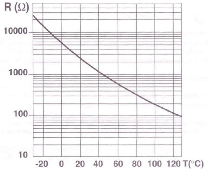
Installed on the water outlet unit, the coolant temperature sensor (thermistor) receives a 5 V supply from the ECU.
