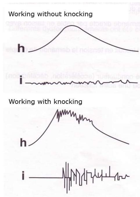
The curve (h) reflects the evolution of the pressure in a cylinder.
