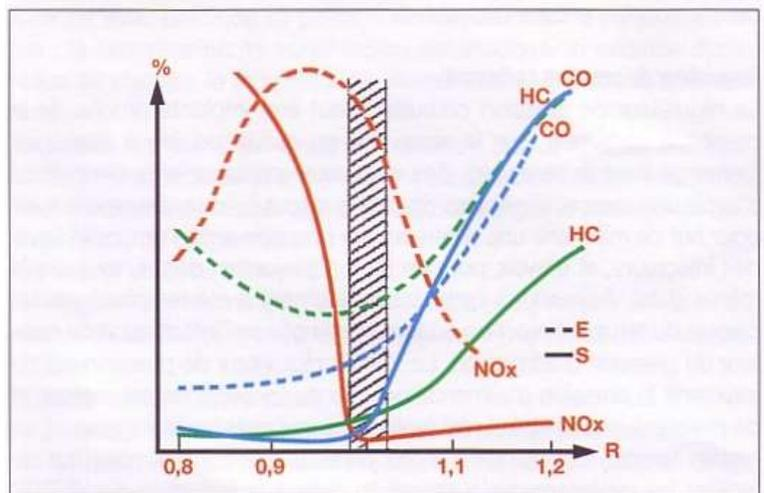
View of the various gases burned during catalysis
