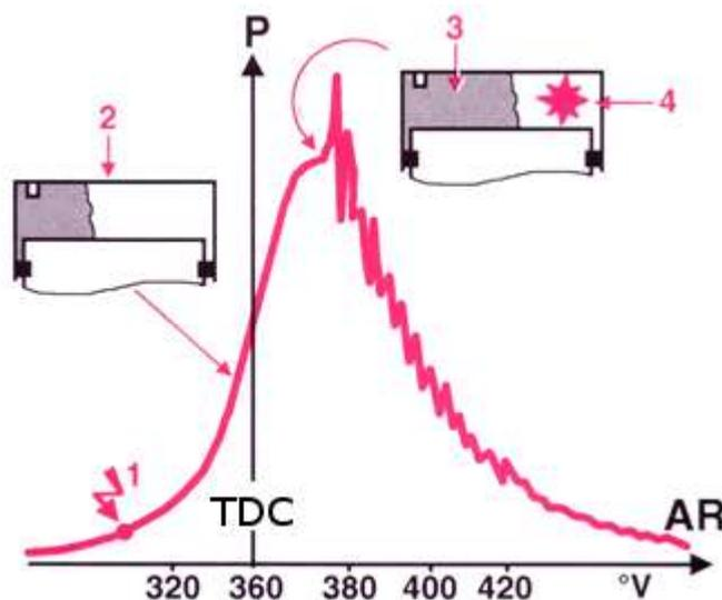
**Pressure diagram in the combustion chamber in the presence of knocking and as a function of the rotation of the crankshaft**
