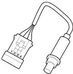
*The oxygen sensor measures the oxygen content of exhaust gases and transmits the information to the ECU as a voltage.*
