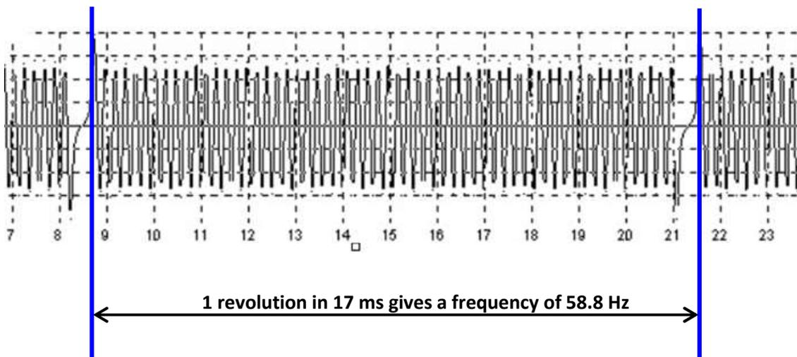
9. Measure the signal from the position/engine speed sensor on the model using an oscilloscope (e.g. REFLET), at a speed of 3500 rpm. Check the accuracy of the engine speed on this signal.
