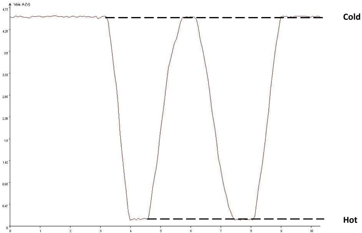
*Graph 8: Double-track accelerator pedal potentiometer*
