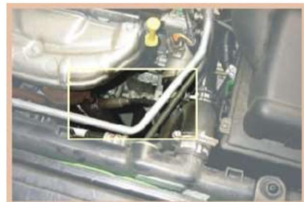
*The sensor is installed on the exhaust line, at the entry to the catalytic converter (upstream).*
