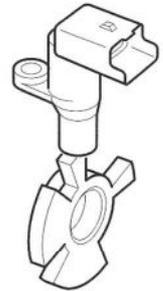
7. How many crankshaft (engine) revolutions are there for a camshaft revolution? Using an oscilloscope (Reflet or CL500, for example), record the phase sensor signal and the engine speed sensor signal then fill in the table
