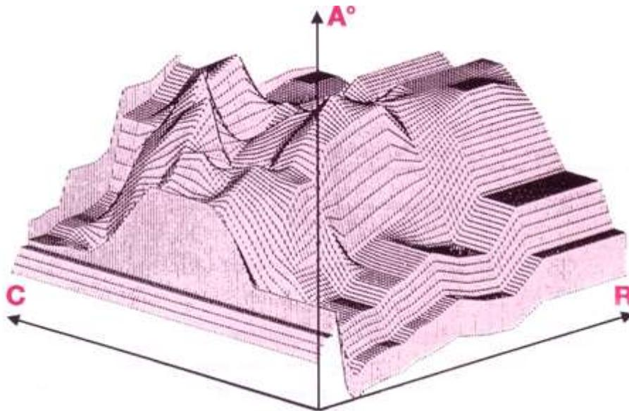
**Mapping of the ignition advance values as a function of the load and engine speed parameters**
