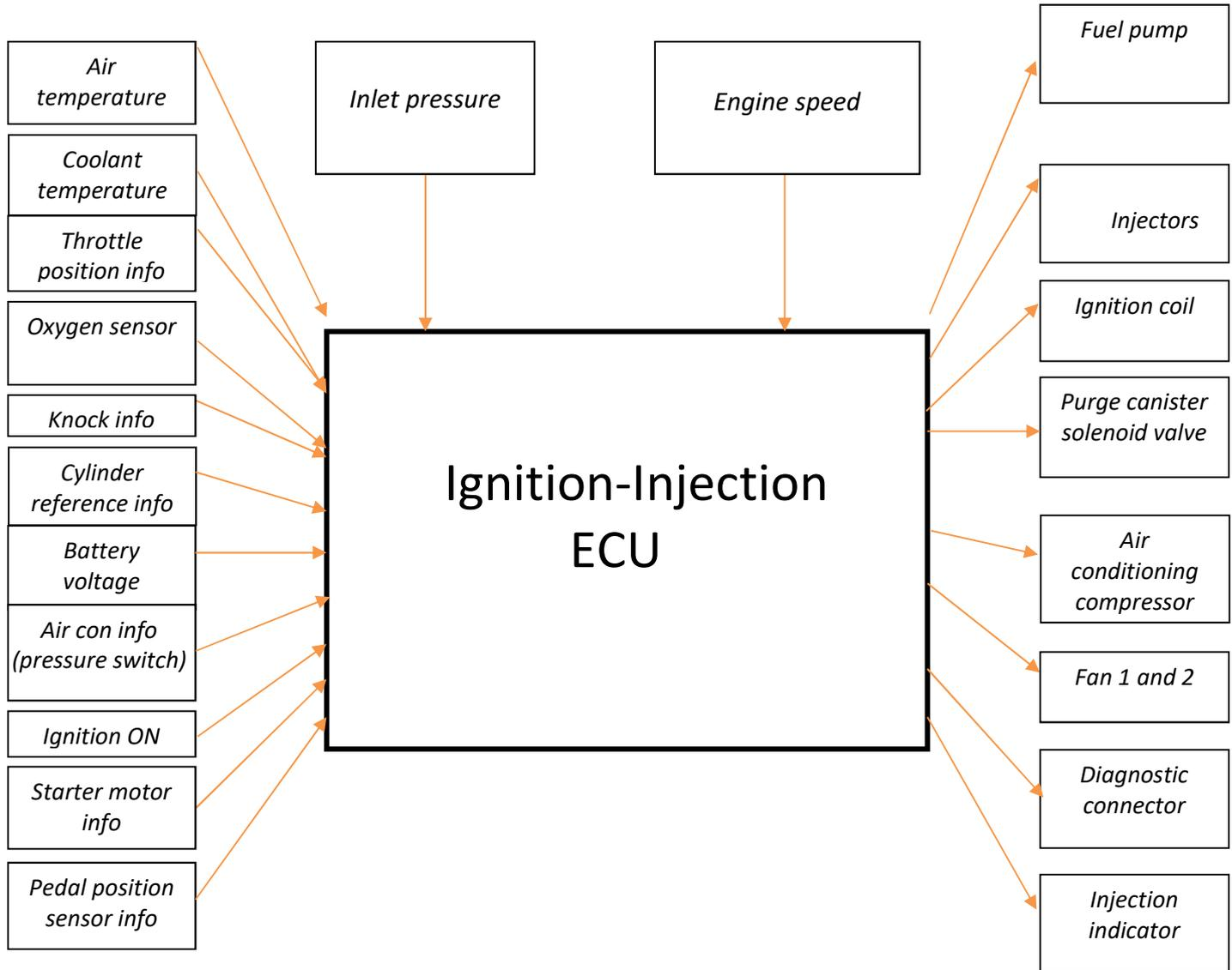
2. ECU input diagram – complete the table
