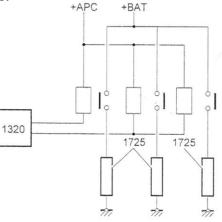
Assembly with two relays - two immersion heater units:
