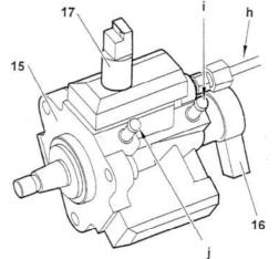
h - high pressure fuel outlet (to high-pressure fuel rail)
