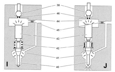
38 - Control solenoid valve ball and needle
