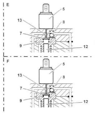
5 - de-activator for the 3rd piston of the high pressure fuel pump
