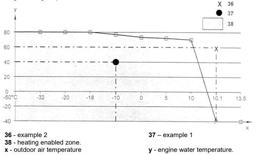
The computer determines heating requirements at start-up depending on the curve.
