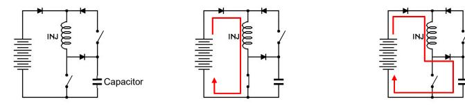
During injections, the capacitor discharges a short-term voltage of 80V into the winding, rapidly establishing a high current and therefore opening the valve rapidly.
