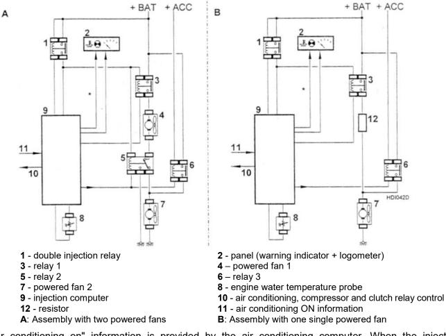
"Air conditioning on" information is provided by the air conditioning computer. When the injection computer receives this information, the powered fans are operated at low speed.
