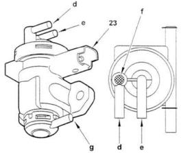
The solenoid valve connects the vacuum pump and the recycling valve capsule for exhaust gases (EGR valve).
