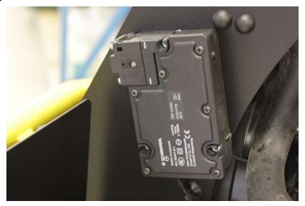
Door security lock, electric opening system, manual closing.
