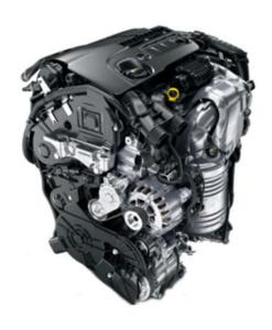
DV6F diesel engine provided by PSA: cylinder capacity of 1600 cm3, turbo, direct-injection « Common rail ».
