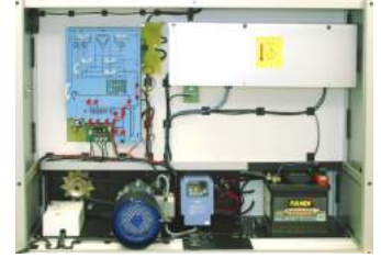
Rear view: battery & charger, electric drive motor
